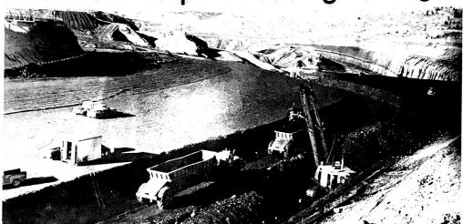
OPEN PIT - Coal mining operations at the Big Horn Coal Company, like almost every mine in Wyoming, use the "strip" mining method
